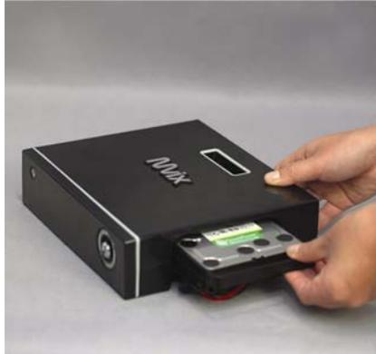
5. As shown above, slowly push the HDD guard together with the SATA HDD into the main body of MvixPVR.
