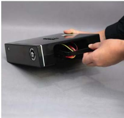
3. Separate the HDD guard from the main body of MvixPVR.
