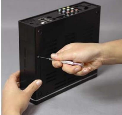
1. As shown above, unfasten the HDD cover screw and open the HDD cover on the side of product.
