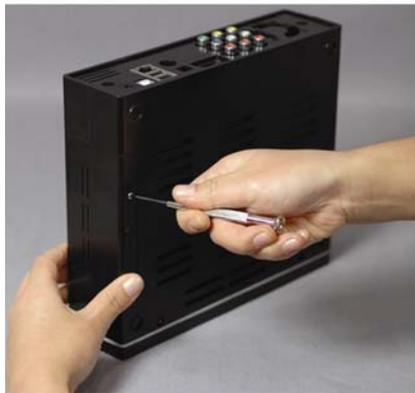
7. When hardware mounting is completed, close the cover and fasten the screw by rotating it in clockwise direction.
