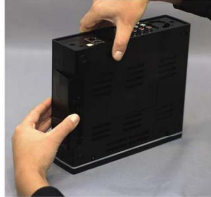
2. Remove the HDD cover on the side of product by pressing it down in the middle as shown in the picture.
