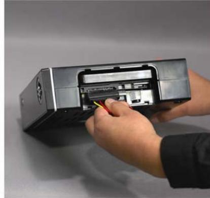
6. Install power cable and SATA cable to the mounted hardware.
