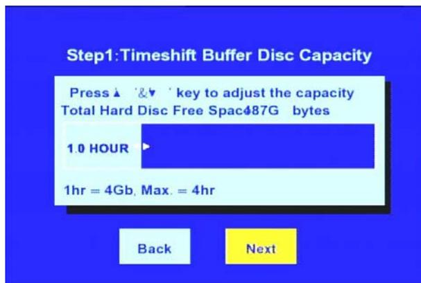
2. The first stage of time shift is adjusted. You can set values by pressing up/ down keys in remote controller. After setup, select 'Next'. Default: 1 hour/ Max. of 4 hours, file system UNIX (UDF)
