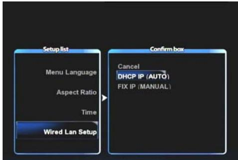
1. Select the method to connect wired LAN to network. DHCP IP automatically allocates IP address.
