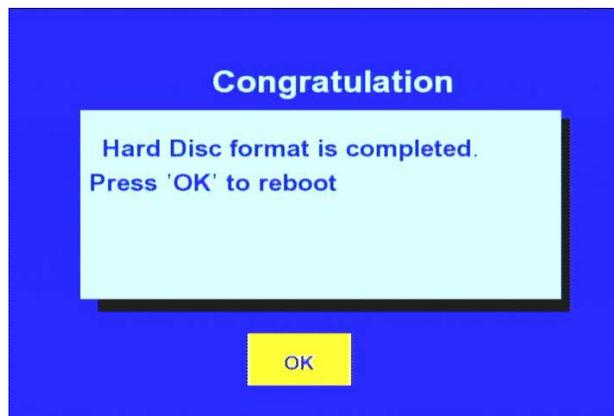
6. When message informing format completion is displayed, press 'OK'. Rebooting is automatically carried out. When rebooting is completed, HDD initialization is completed.
